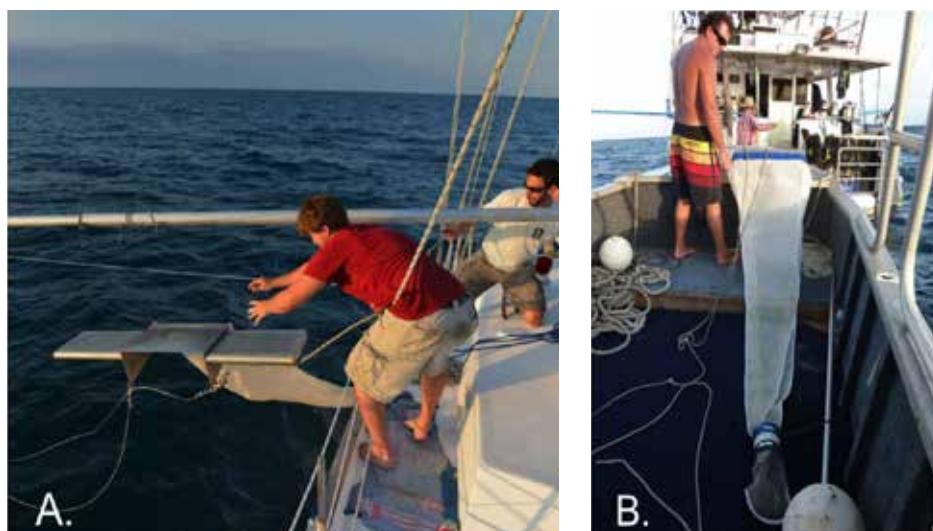
Figure 5.3. The manta trawl has wings and can float unassisted (A). The neuston net must be suspended at or below the water's surface (B).
