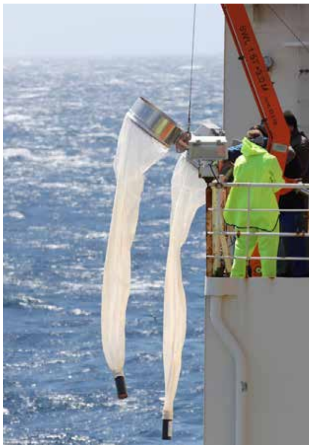
Figure 5.5 The Bongo net captures sub-surface microplastics.
